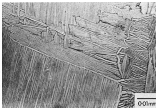
Figure 6 Ti 1 wt % Mo 1100°C/10 min furnace cooled. Light micrograph showing \alpha phase outlining the prior \beta grain boundaries and a lamellar mixture of \alpha and \beta phases within the grains ( \times 800 ).
